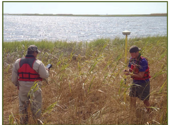
LSU Coastal Engineering Ph.D. student, Kyle Parker (right) and T Baker Smith LLC's employee surveyed the marsh elevation in Breton Sound during sensor retrieval on September 11, 2012.
