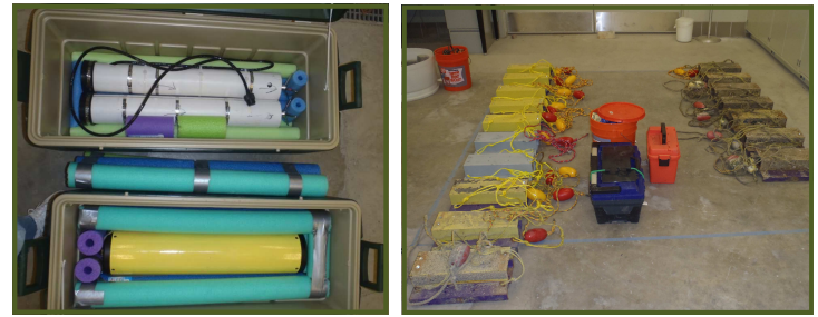
Wave and surge gages in Chen's coastal engineering lab at LSU before deployment.
