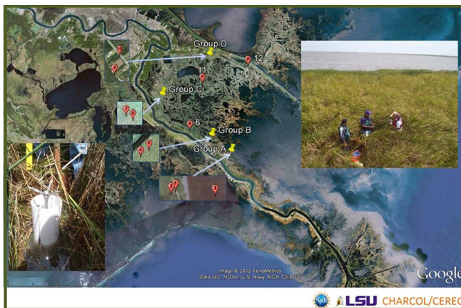
Locations of wave gages (Groups A-C) and surge gages deployed by Chen's group at LSU on August 27, 2012 prior to Hurricane Isaac's landfall on the Louisiana coast. Right inset: Kyle Parker (left), Ranjit Jadhav (middle) and Arash Karimpour (left) installed wave gages on the marsh.
